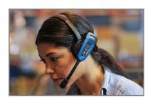
The Vocollect SRX2 wireless headset provides an embedded multi-microphone array to reduce unwanted word and sound insertions by more than 50% compared to other headsets used in the distribution center. It uses high fidelity acoustic sampling for higher audio clarity.
